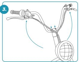
Adjust Handlebars to Desired Position
