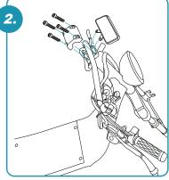
LED Display Align the LED display mount holes with the front bracket mount holes. Attach loosely with 4 screws.
