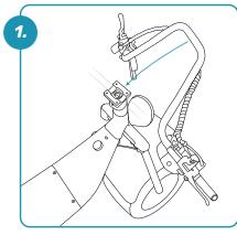
*Handlebars* Place handlebar on bottom bracket notch.
