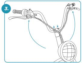
Adjust Handlebars to Desired Position Find center and correct height. Hold in place while screws are tightened.
