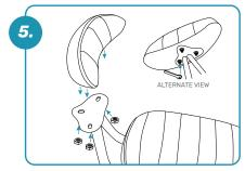
*Rear Seat* Place seat on rear support bracket. Hold in place, fastening each of the 3 nuts until tight.
