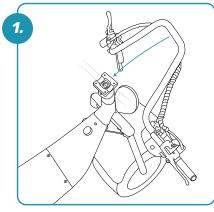
Handlebars Place handlebar on bottom bracket notch.
